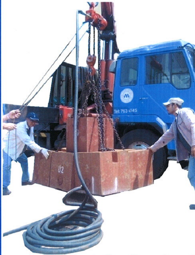
Load Test for Overhead Crane / Hoist
